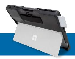
In an office environment, a CAC reader is typically a standalone peripheral connected to a USB port on the desktop, laptop, or tablet. Because the BlackBelt integrates the same form of card reader into its case, users on the go do not need to carry a separate peripheral with them and will immediately recognize how to use it.
